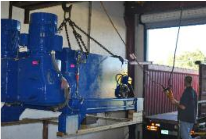
CM Primary Shredder being loaded into open top container
