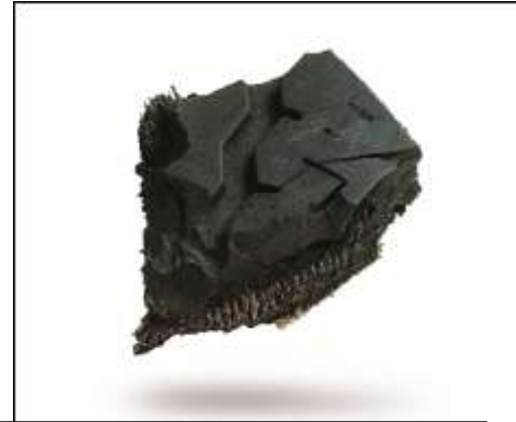
A CM Tyre Shredder produces a 50 mm clean cut tyre chip, ideal TDF for cement kilns.
