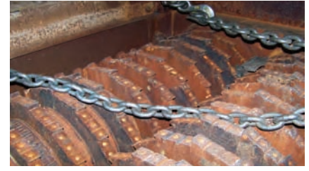
Geocycle's Dual Speed Shredder cutter box and assembly being loaded on a flatbed on its way back to CM for a complete rebuild.
