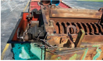
Geocycle's Dual Speed Shredder cutter box and assembly being loaded on a flatbed on its way back to CM for a complete rebuild.
